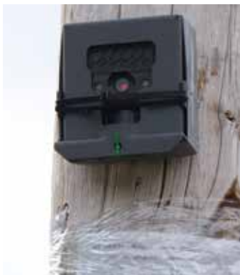
One of the automatic cameras set on a pole in Kangiqsualujjuaq to observe snow-avalanche occurrence.
