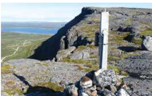
An automatic camera set on the top of the plateau above Tasiapik Valley near Umiujaq, to observe the snow-cornice formation, that triggers snow avalanches while collapsing.
