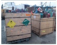
An example of how to properly package a crate containing empty gas cylinders.
